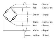
Shield connected to load cell body
